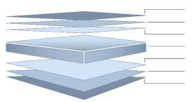
Finish Coat (Finish Coat + Primer = nominal 19µm) {Refer Notes 3 & 4} Universal Corrosion Inhibitive Primer Conversion Coating Aluminium / Zinc / Magnesium alloy-coated steel with Activate<sup>®</sup> technology substrate Conversion Coating Universal Corrosion Inhibitive Primer
